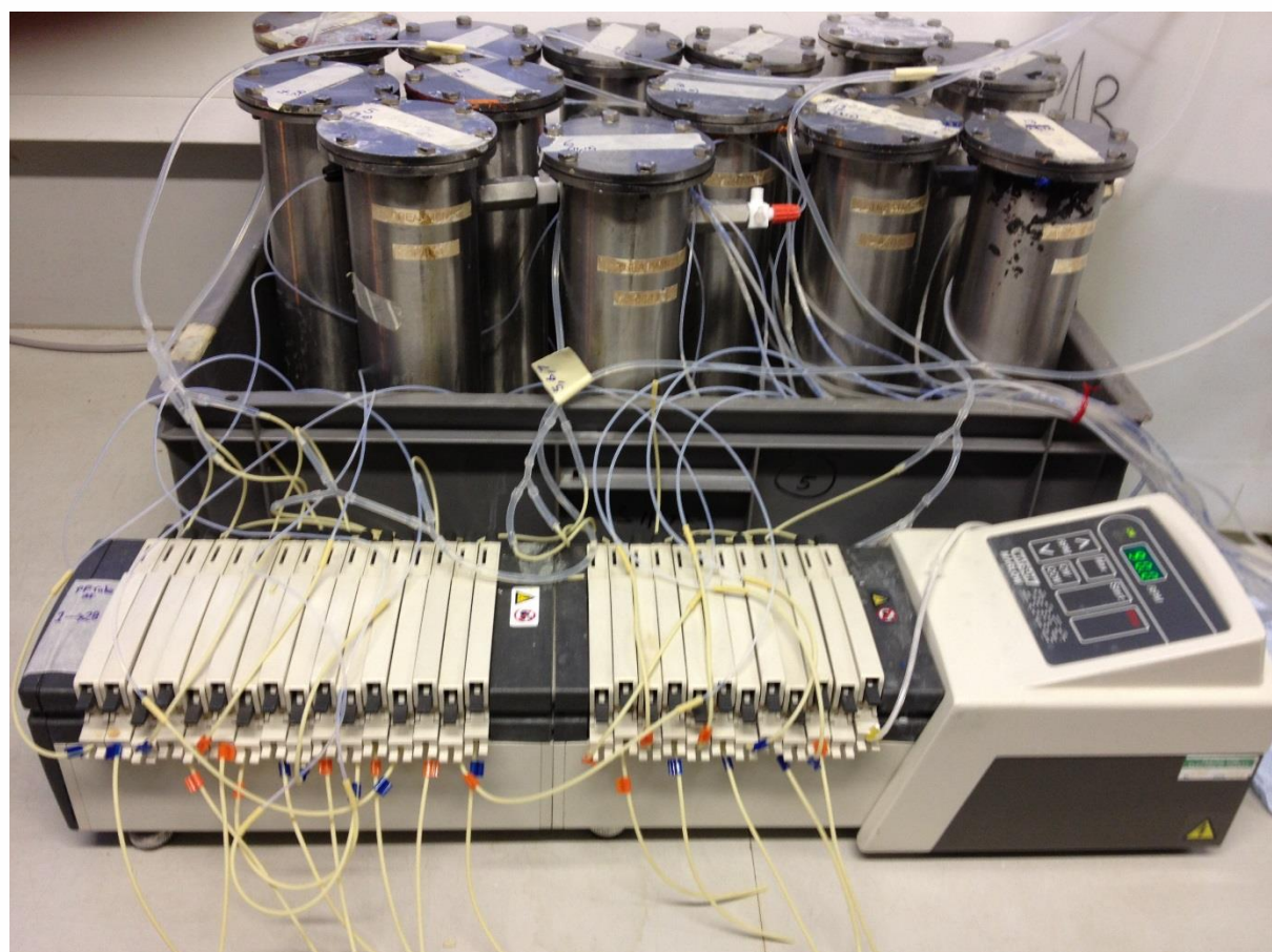
Figure 2 – Leaching columns setup
